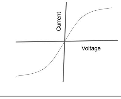
A filament lamp. As the current increases, the resistance also increases. This means that the gradient will decrease as current increases.
