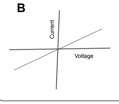
B has a shallower gradient, and as the gradient=1/R, a smaller value for the gradient = a higher value for the resistance. A higher voltage is required in B for the same change in current in comparison to A.
